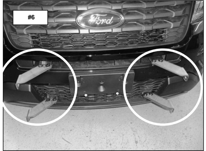
**Step-8** Attach the push bumper to each of the extension brackets using (2) 3/8" x 1" hex bolts, (2) 3/8" lock washers and (2) 3/8" hex nuts, (Photo 7 & 8). Leave the nuts and bolts loose for final adjustment.
