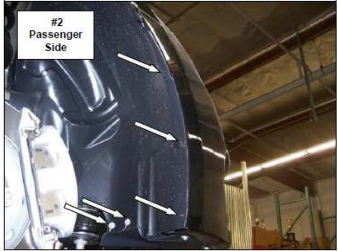
3. Pull back the fender liner and remove the Phillips screw and plastic fastener attaching the fascia to the fender. **Picture #3**
