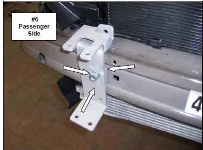
3. Insert the top of the passenger side clamp bracket through the gap between the impact beam and auxiliary cooler, and then rotate the bracket into position. Slide the bracket to the left and align the holes in the clamp bracket with the main bracket. Secure the clamp bracket to the main bracket using (2) 3/8" x 1" carriage bolts, (2) 3/8" lock washers and (2) 3/8" hex nuts. **Picture #7 & #8** Leave the nuts and bolts loose for final adjustment.
