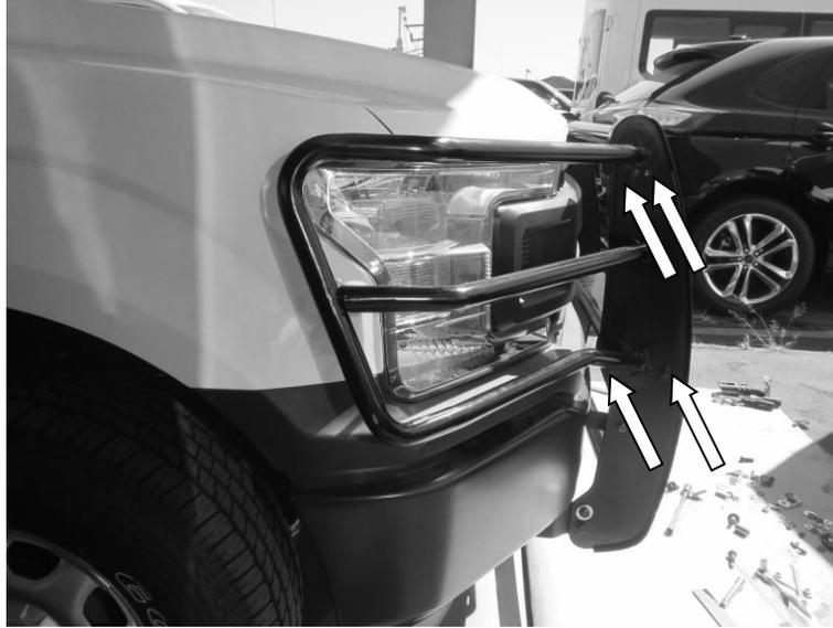
3. Align the push bumper and brush guard assembly and tighten all nuts and bolts securing the push bumper, brush guard assembly and brackets, (Photo 2).
